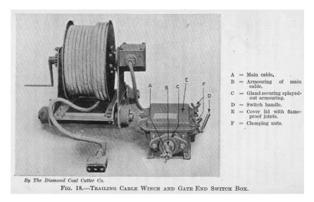
These gate end switch boxes are constructed very solidly, and, given reasonable care, they should never cause any trouble. The main cable is shown at A, the three cores being shown separated; the armouring B of the main cable is held firmly to the gate endswitch box by the gland and clamp ( $\sim$ . The switch handle D cannot be operated unless the lid E is closed and secured tightly by the clamping screws FF.
