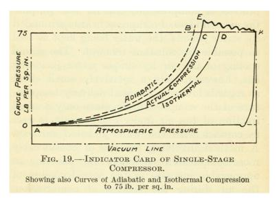
Fig. 19 shows the curves of adiabatic and isothermal compression of air to a pressure of 751bs. per sq. in. In practice, the indicator card of an air cylinder of a compressor shows a line intermediate between these two curves, the actual compression curve being very near the adiabatic curve when the cooling has only a small effect, and approaching nearer to the isothermal curve when the effect of cooling during compression is at a maximum.
