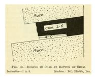
In Fig. 15 the holing is extremely hard and the material very close-grained. The total thickness of the fireclay under the coal is from 8 to 10ins.; the machine takes out the top 5 to 6ins. of the underclay and the dirt left on by the machine forms a 'bench' which facilitates the cutting by preventing holings from being churned up by the disc and carried back into the cut. This bottom dirt is got up by the colliers when the coal is filled out.
