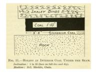
In Figs. 11, 12, 14 and 16 the positions of the bands of dirt or of inferior coal were the deciding factors in determining the position of the cut. In Fig. 13 the coal parts fairly easily from the roof but
